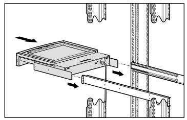
Figure 2-6. Inserting the retractable tray into the rack
